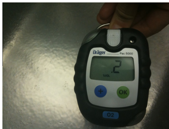
Figure 4 Oxygen check. Before LN 2 (liquid nitrogen) sterilization the presence of oxygen in the environment at 15 cm from LN 2 surface was checked by using a portable oxygen detector (Pac 5000; Dräger, Lübeck, Germany). The nitrogen vapour phase resulted virtually free from oxygen (less than 0.2%) at every check.
